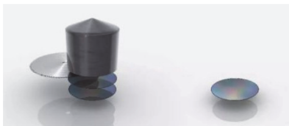
图2 硅棒和硅晶圆片 [2]
